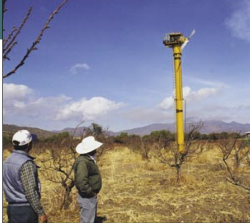
José Luis Acevedo (left) and a visiting farmer watch a wind machine installed to control frost in a peach orchard in Jerez.
